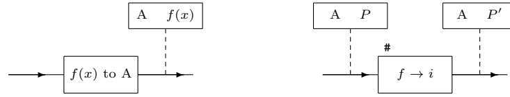
Fig. 5. Conditions on storage boxes preceded by operation (left) and substitution (right) boxes. The configuration on the right must satisfy the condition P'[f \rightarrow i] = P
